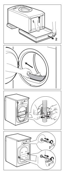
Remove the polystyrene protection from the bottom. Pull up the appliance in vertical position.
