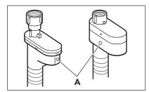
The inlet hose has a water stop device. This device prevents water leaks in the hose because of its natural ageing.
