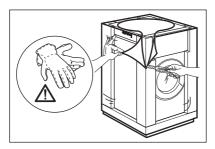
Use the gloves. Remove the external film. If necessary, use a cutter.
