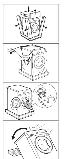
Remove the cardboard top. Remove the polystyrene packaging materials.
