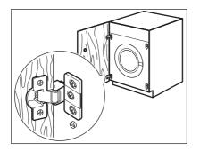
The appliance is originally pre-arranged for the assembly of a door opening from right to left.
