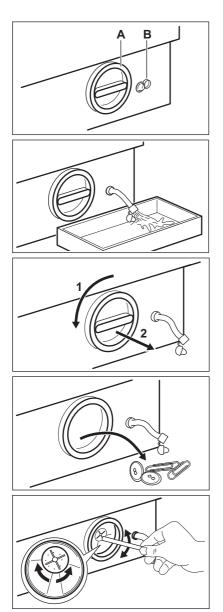
3. Place a container close to the pump to collect any spillage.
