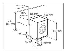
This appliance has been designed to be built into the kitchen furniture. The recess should have the dimensions shown in this picture.
