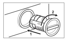
8. Put the cap back on the emergency emptying hose and place the latter back in its seat. Replace the filter into the pump by inserting it correctly into the special guides. Screw the filter cover firmly by turning it clockwise.
